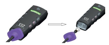
Fig. 3 Replacing Probe Filter
